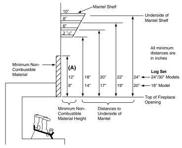
Figure 6 - Minimum Mantel Clearances Without Using Hood
